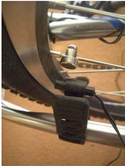
Magnet on wheel spoke, sensor on trainer frame
