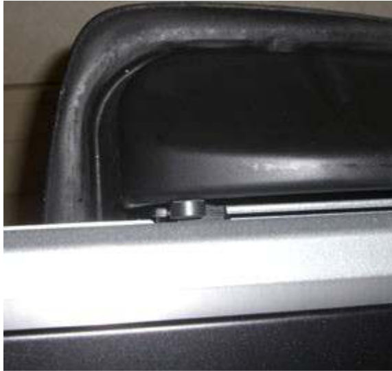
Wheel magnet on seat of rowing machine
