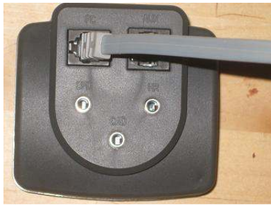
Serial cable plugged in PC jack of ITS Box
