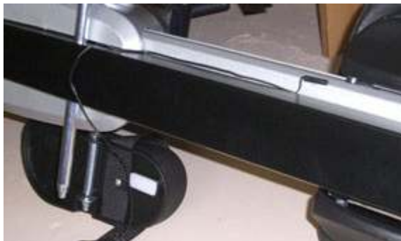
Speed sensor installed along machine frame
