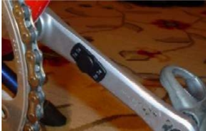
Wheel magnet on pedal arm of exercise bike
