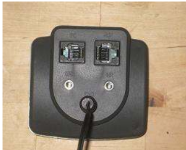
Sensor plugged in CAD jack of ITS Box
