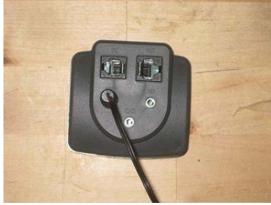
Sensor plugged in SPD jack of ITS Box
